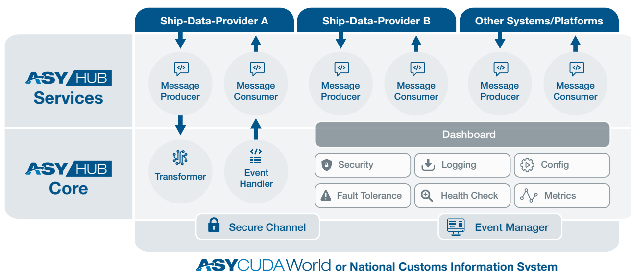
Figure 5: ASYHUB global technical architecture
